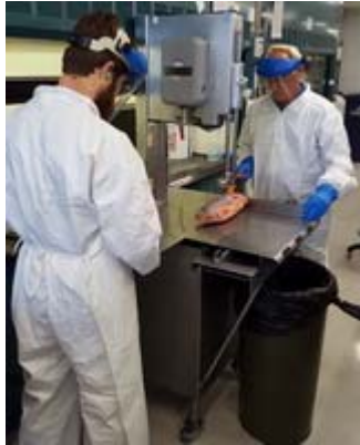
Ronald Kulwicki is a Lab Technician and in this photo is band sawing large fish samples from Michigan waterways to prepare them for extraction and determine if they are contaminated with mercury or pesticides.
